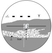
Recommended Distance Mode (indicated by RD and ✓ icon in viewfinder) adjusts distance based on angle of the slope. Aim, then press and release top ( button. Distance and slope angle readings will alternate in viewfinder. (This mode also includes MG-Lock. indicated by icon, which locks
